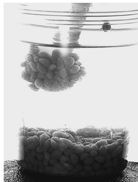
Fig. 5 Magnetic iron-encapsulated wet cellulose beads
